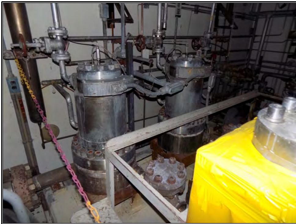
Figure 78. Current photograph of pressurized-water loop experimental facility located in the westernmost Irradiation Engineering Room on the north side of the basement in Building 3042.
