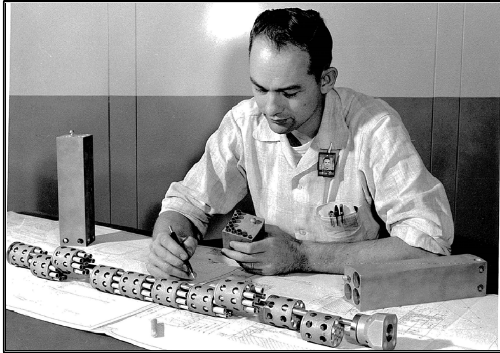
Figure 198. Archival photograph showing an ORR Isotope Irradiation Assembly, circa 1957. Isotope cans were inserted into the cylindrical chambers prior to the assembly being inserted into the ORR for irradiation (ORNL Photo 41741) (Neumann 1961:6).
