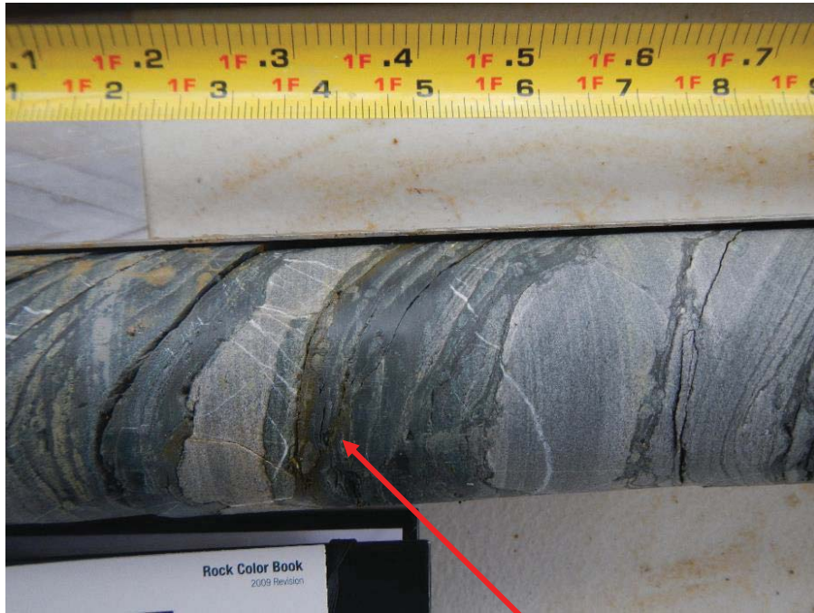
GW-989 30.0' – 45.0' Sand Pack Interval 33.6' – 43.6' Screened Interval April 2018
