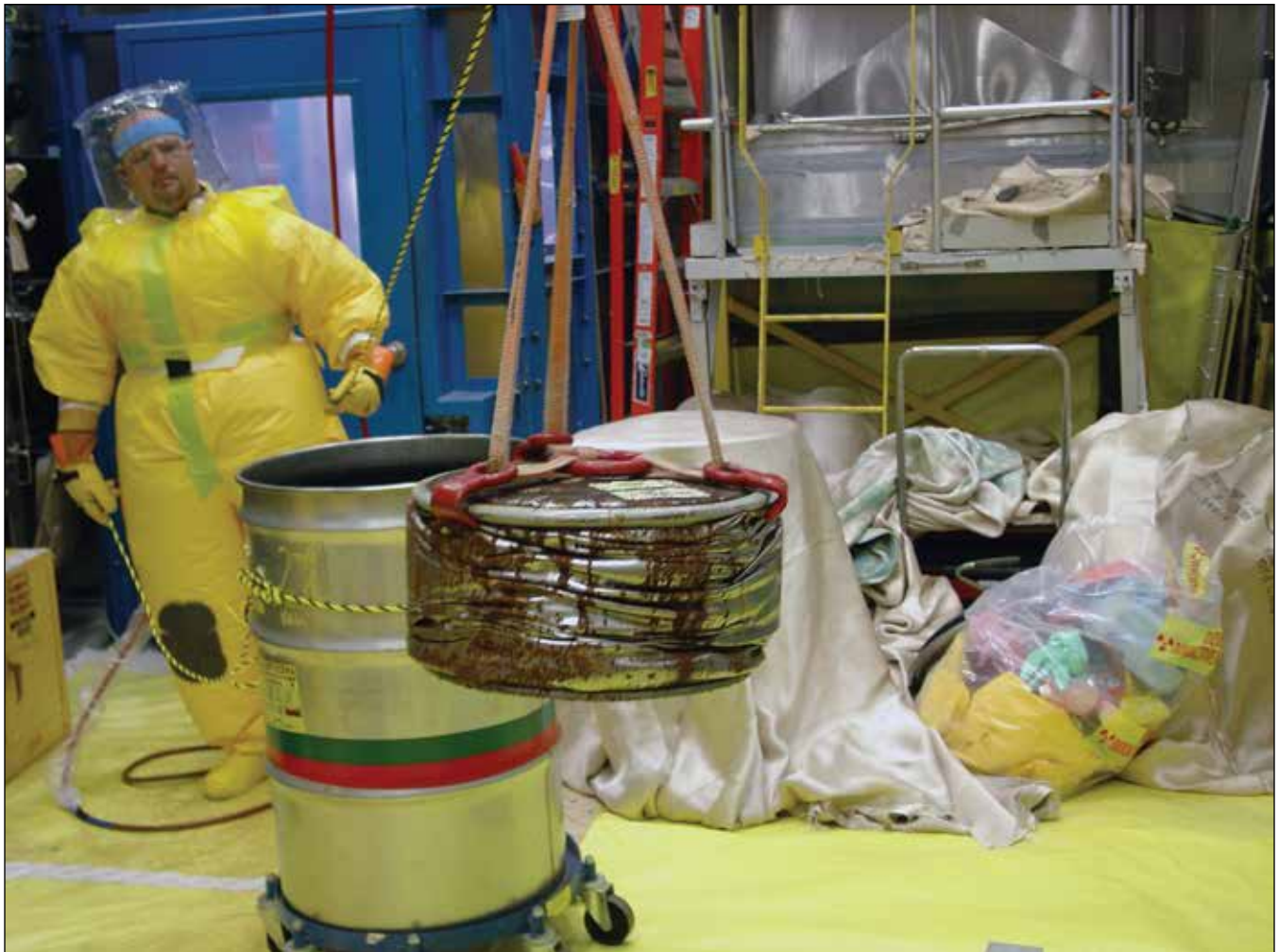
A TWPC worker removes a supercompacted waste puck from 55-gallon waste drum
