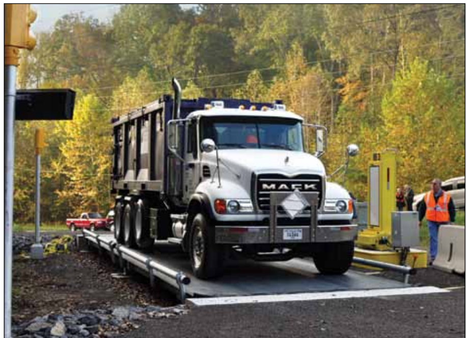
The RFID tower (yellow device) reads the shipping information on trucks.
