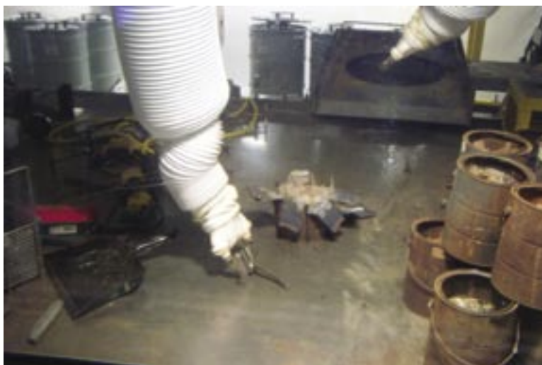
Cans of RH-TRU waste being processed in the Hot Cell
