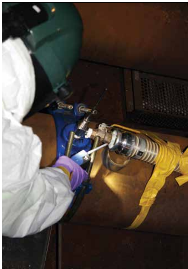
A technician samples gases vented from a process gas system to verify the absence of hydrogen fluoride.
